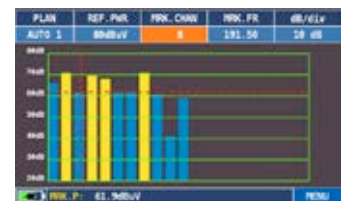
BAR Scan showing both Analogue and Digital Channels
