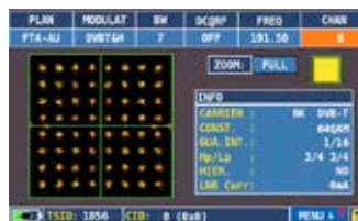
Terrestrial Digital Constellation Measurements
